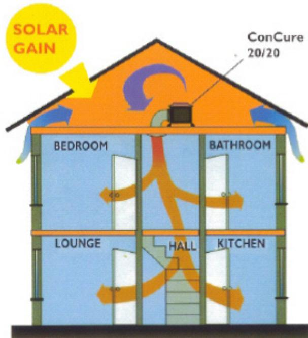
Positioned in the loft above the landing or the central hallway of a bungalow, the system takes maximum advantage of solar gain.
